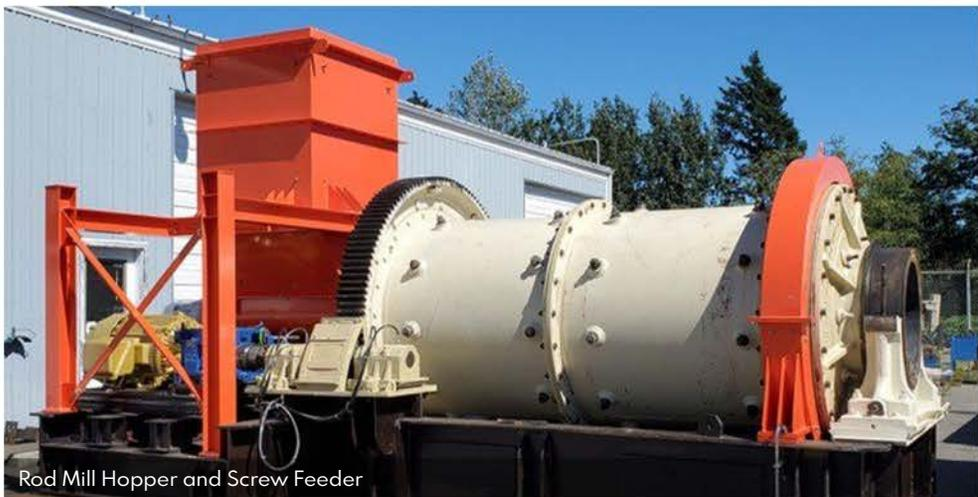
Rod Mill Hopper and Screw Feeder
